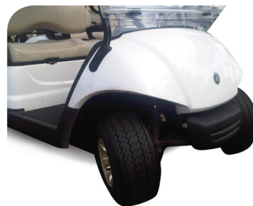
Golf Car Parts Acrylic Capped ABS - Body formed on a Formech 1500
