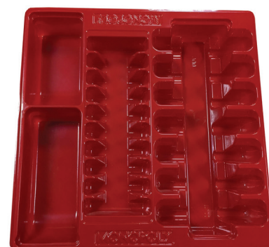
Monopoly board game - Vacuum formed on a Formech 686
