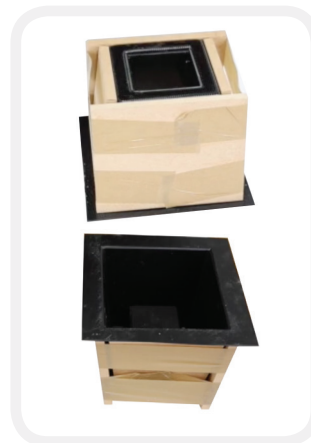
The outer faces of the vacuum forming are strengthened with MDF panels and attached with double sided tape. All the MDF panels are then secured with packaging tape to stop the panels from moving.
