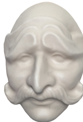
Mask DUESITH - Body formed on a Formech 300XQ
