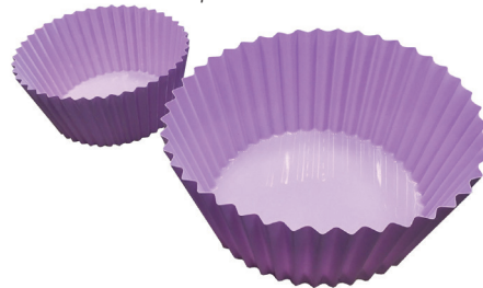
Cup cake POS display - Body formed on a Formech 686
