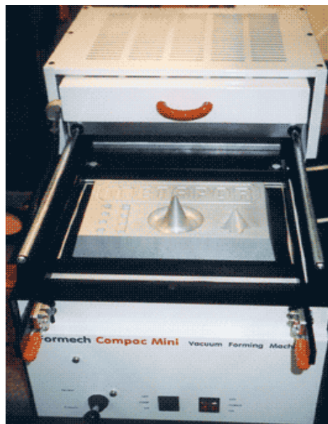
Fig. 5.4 A metaphor mould demonstrated on one of the Formech range of vacuum forming machines
